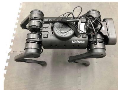
A1 Robot with speakerphone installed
