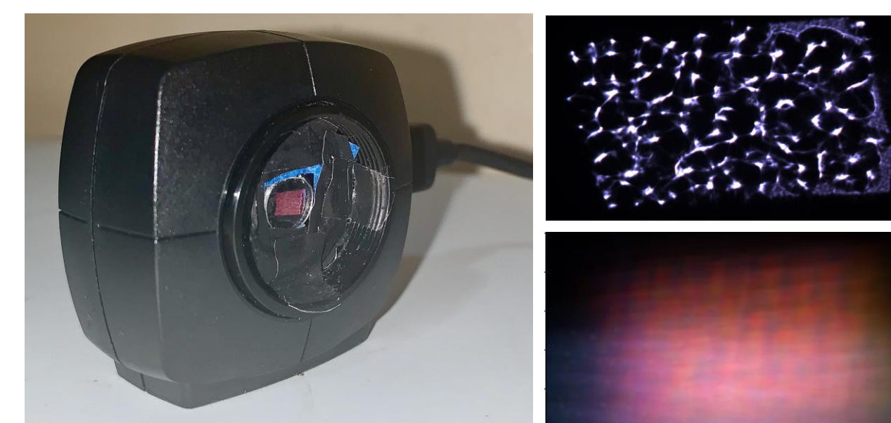
Experiment image: Lensless camera with its PSF and a sensor measurement of a Rubik cube
