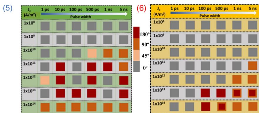
**Dynamics:** Switching map depicting the effects of pulse amplitude v. pulse width. (5) Current injected through the HM/AFM system. (6) Current injected through the HM/AFM/FM system.
