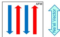
**Antiparallel** magnetic moments in AFMs result in no net magnetization in the system. Ne'el vector points parallel to AFM spins.
