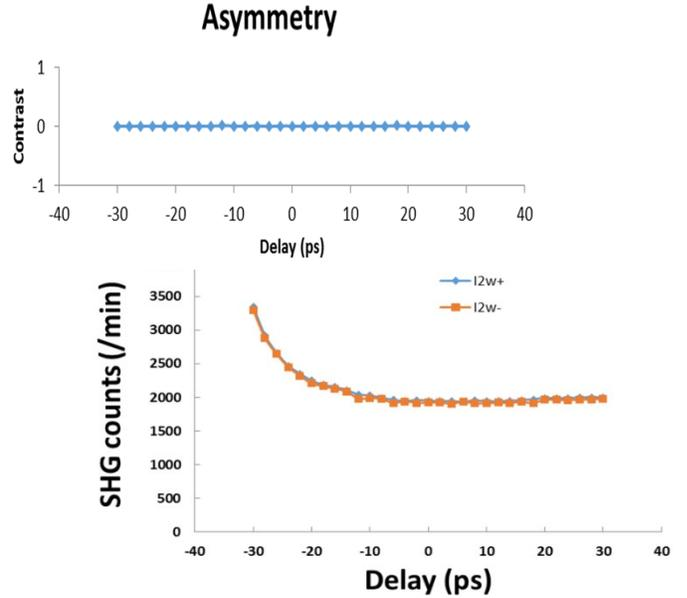
the higher the magnet moment of the heavy metal. However, my results showed no contrast of spins. Figure 3 shows that my Asymmetry values were zero for each delay point in the current pulse and the identical number of spins in the positive and negative orientation.
