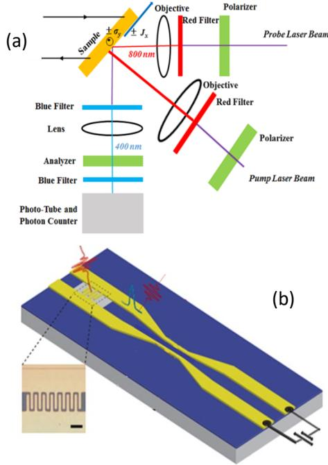
being positioned through the imaging optics thus the red filters are to cancel out any other signal from coming in contact with the sample. The blue filters are to block any signal other than the second harmonic from being measured by the photo tube.
