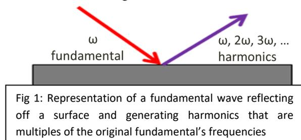
Fig 1: Representation of a fundamental wave reflecting off a surface and generating harmonics that are multiples of the original fundamental's frequencies
