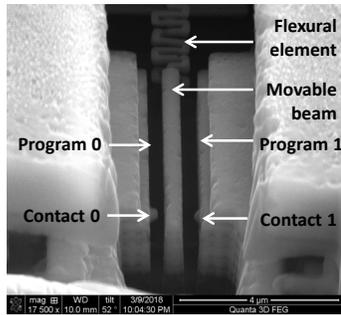
Figure 3: Cross section SEM of NEM device
