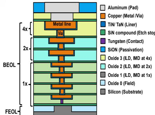
Figure 1: BEOL Process Cross Section used to fabricate the NEM reconfigurable interconnects
