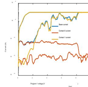
Figure 6: Current-voltage characteristics showing reprogramming for the NEM interconnect
