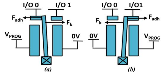
Figure 2: Schematic of NEM reconfigurable interconnect when (a) programmed to state “0” and (b) reprogrammed to state “1”
