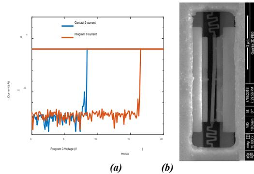
Figure 5: Catastrophic pull-in: (a) current-voltage characteristics and (b) SEM image
