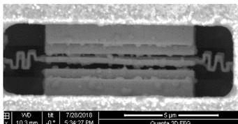
Figure 4: SEM of NEM interconnect with etch by-product on sidewalls
