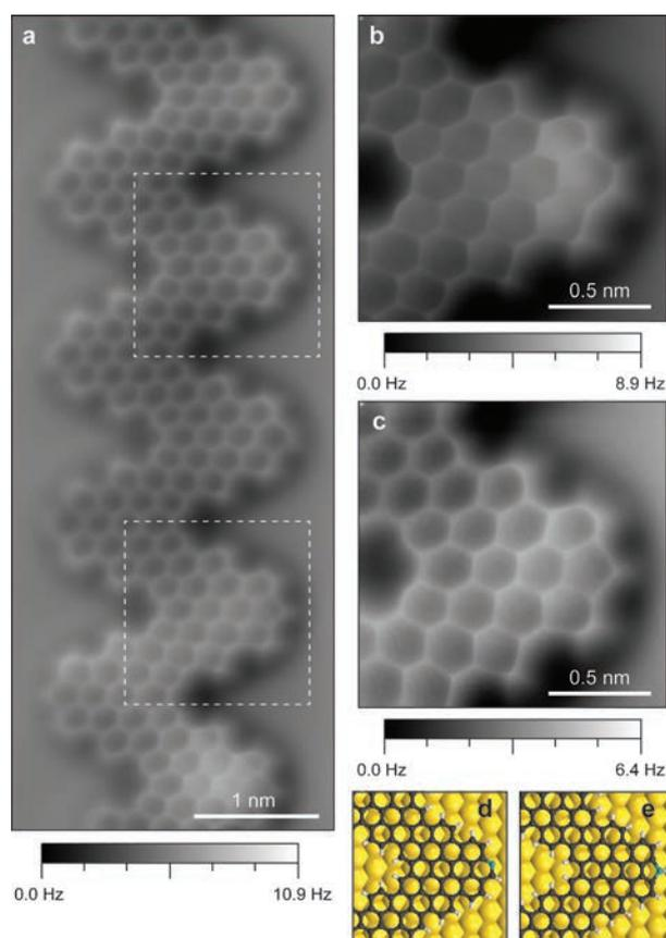
**Figure 3.** a) nc-AFM image (CO modified tip) of chevron GNR heterostructure on Au(111) featuring discrete segments of fused phenanthridine and carbazole groups (qPlus resonance frequency = 23.17 kHz, oscillation amplitude = 56 pm). b) nc-AFM image of phenanthridine-fused GNR segment. c) nc-AFM image of carbazole-fused GNR. d), e) Ball and stick model of phenanthridine- and carbazole-fused GNRs serves as a guide for the eye.
