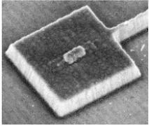
❑ Electrical injection III-V antenna-LEDs
