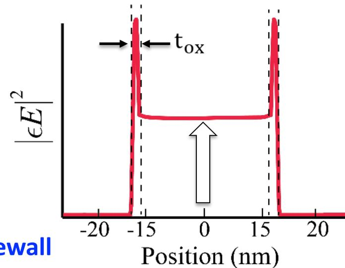
Oxide thickness on sidewall reduced from 3 nm to 1 nm
