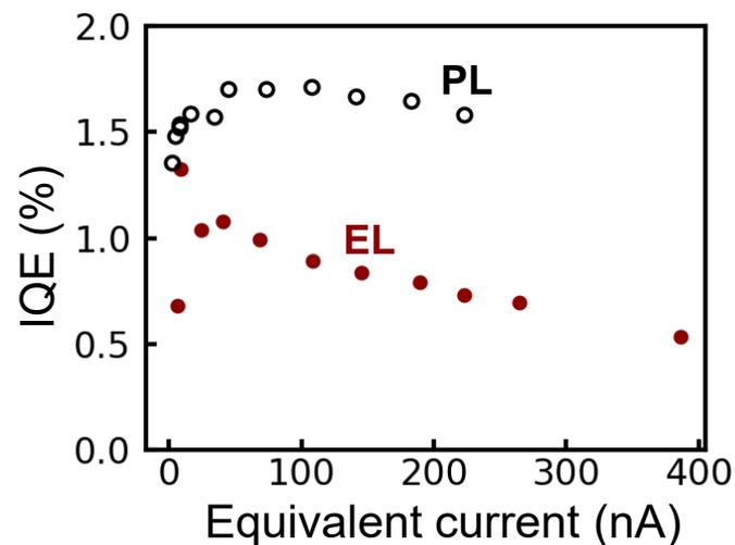
Process improvements yield EL efficiency close to PL (~1%), indicating material-limited efficiency
