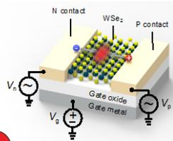
❑ Monolayer TMDC antenna-LEDs
