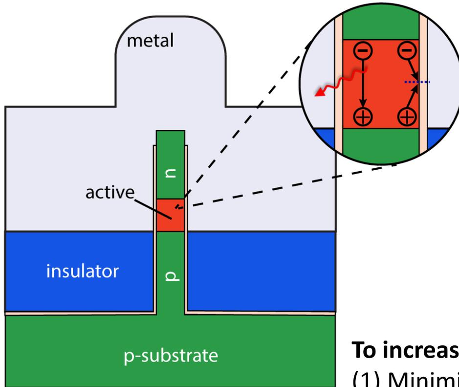
$$I_{tot} = \underbrace{AN}_{I_{nr}} + \underbrace{BN^2}_{I_{rad}} + \underbrace{CN^3}_{I_{Auger}}$$
