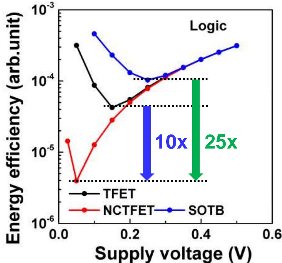
Negative capacitance can boost  $I_{on}/I_{off}$  of TFET and improve energy-efficiency by 10X.
