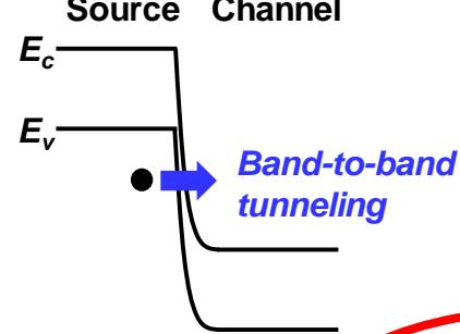
$$SS = 2.3 \frac{k_B T}{q} \left( 1 + \frac{C_d}{C_{ins}} \right)$$
