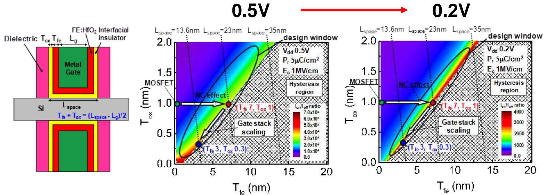
**Very thin FE-HfO<sub>2</sub> gate stack can fit in advanced gate last process, with steep slope.**
