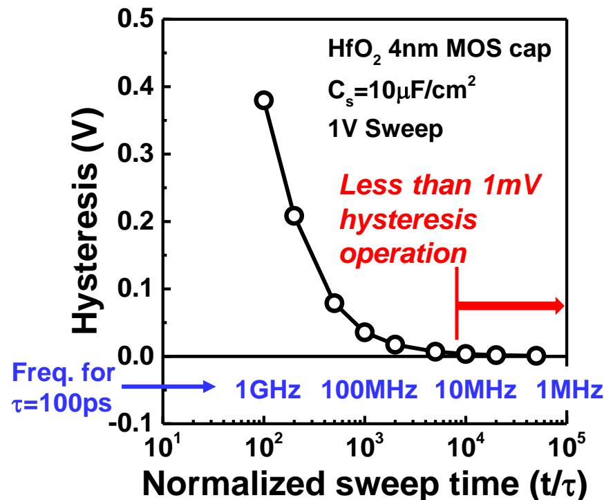
Suppose  $\sim 100\text{ps}$  time constant, NCFET can operate at  $>10\text{MHz}$  without hysteresis.
