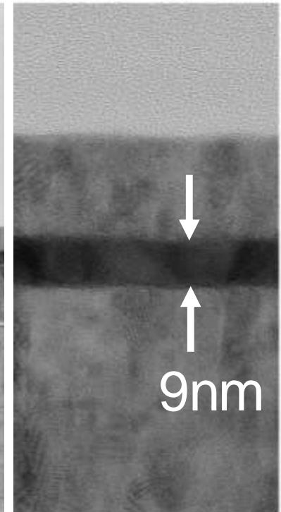
Prototype NVSRAM was fabricated in university's lab integrating FE-HfO<sub>2</sub> on CMOS SRAM
