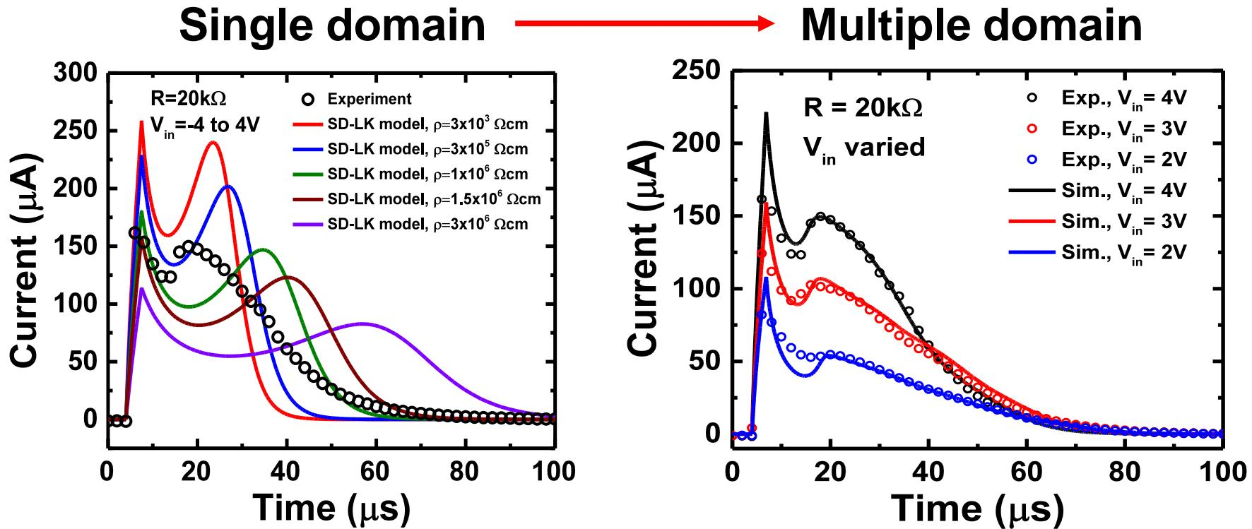
Multiple domain model improved fitting accuracy to experimental data.
