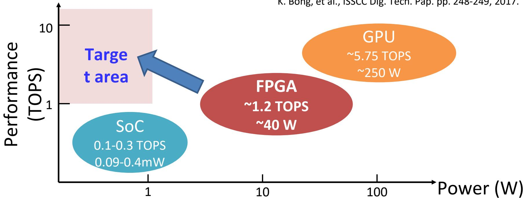
**FPGAs** is a key device to realize “energy-efficient” hardware.
