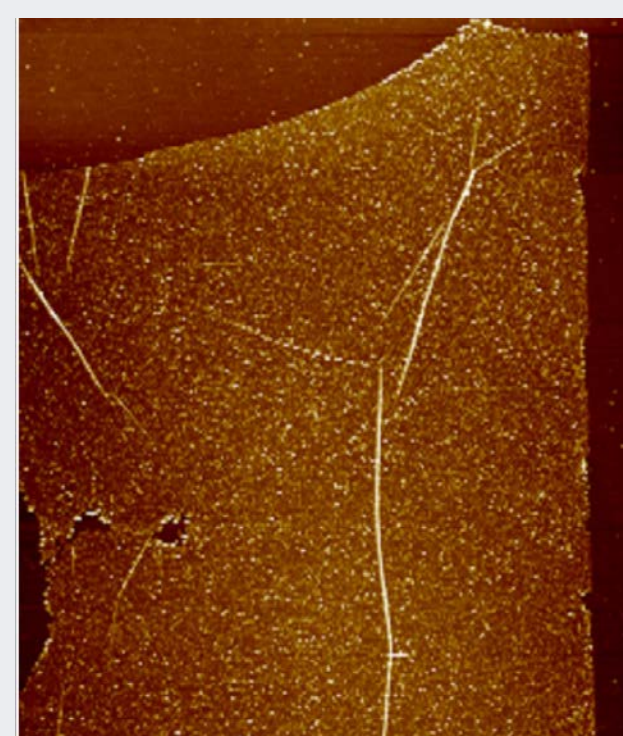
AFM image of flake before Au NPs decoration
