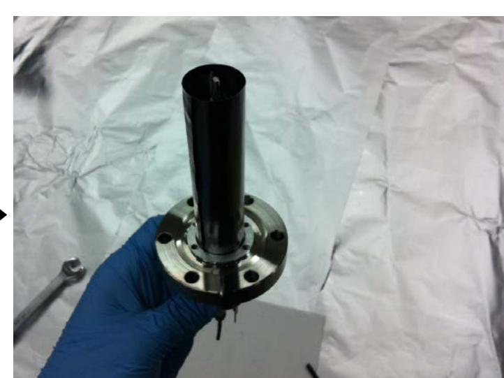
Fig. 4: Copper Heat Shield
