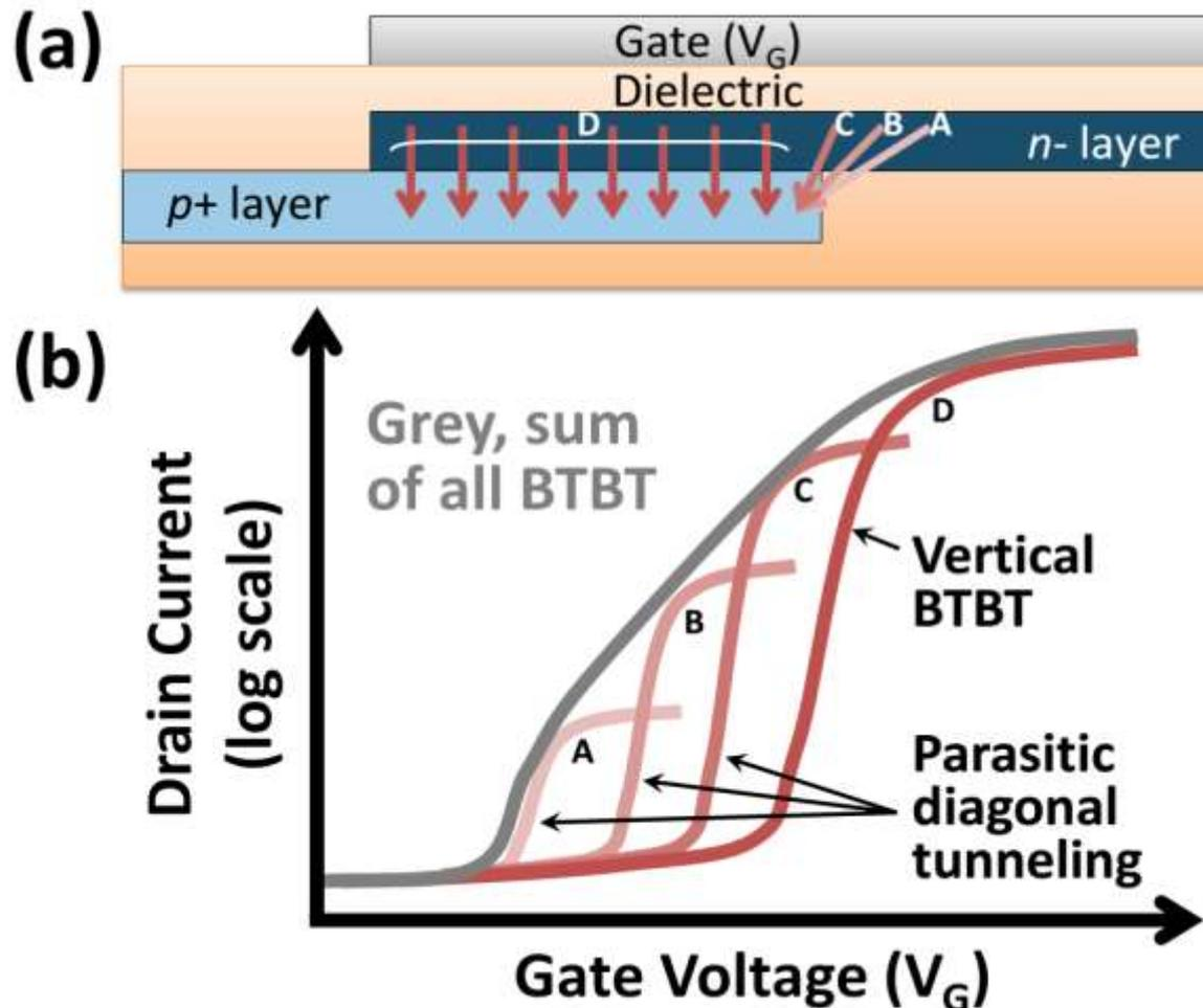
Though **D** is the desired tunneling path, parasitic paths **A-C** significantly reduce the sharpness of the turn-on (akin to varying threshold voltage).
