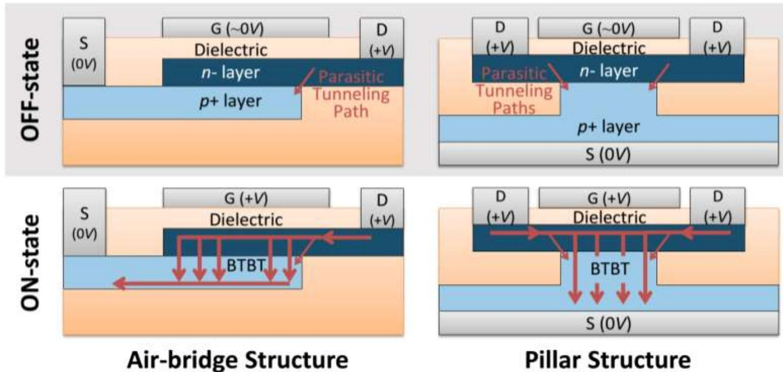
Parasitic diagonal tunneling paths can limit the off-state AND degrade the switching performance.
