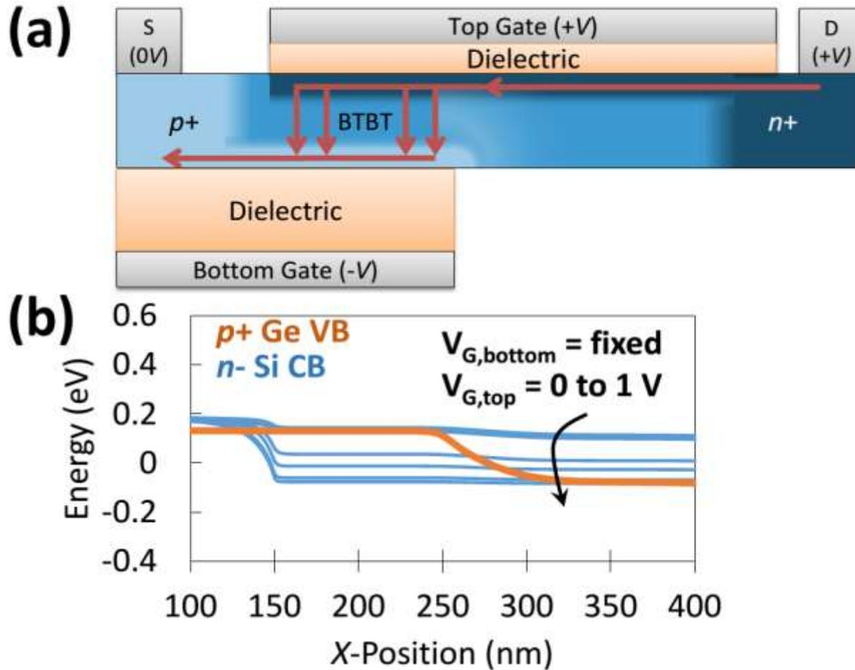
Lateral electric field can be greatly reduced using thick bottom oxide
